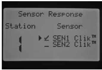
Sensor 1 only programmed for Station 1
