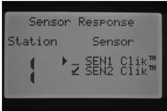
Sensor 2 only programmed for Station 1
